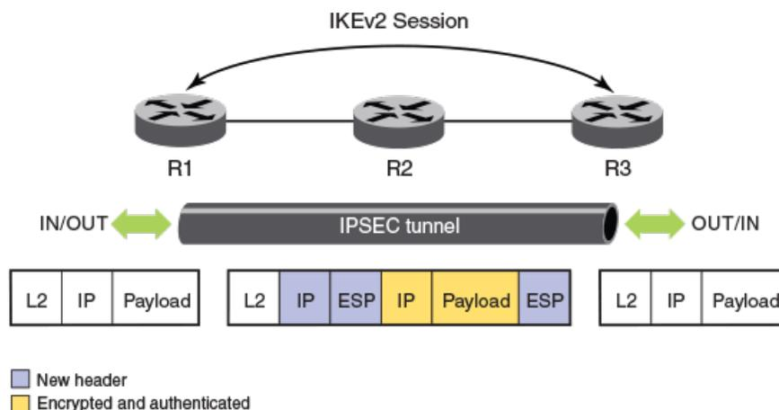
The preceding figure shows the secure transfer of IP data between two routers, R1 and R3, over an insecure or public network by using IPsec. First, the tunnel parameters, transform set, and crypto algorithms to be used for encryption and authentication along with associated policy filters are configured on both R1 and R3. IKE negotiations are used to establish the tunnel.
