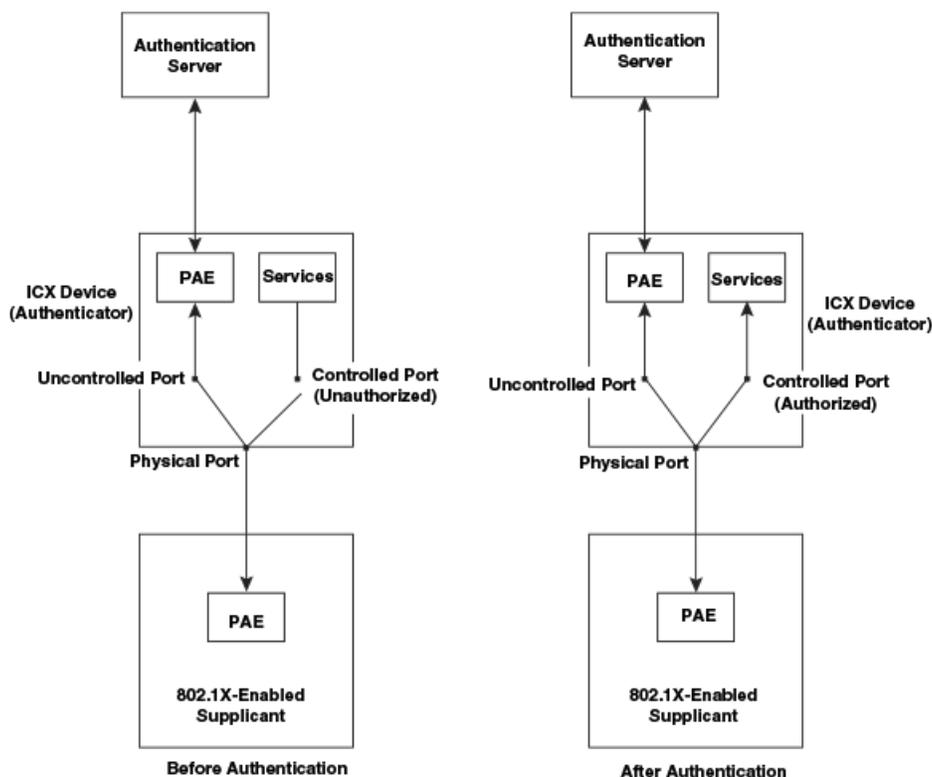
Before a client is authenticated, only the uncontrolled port on the authenticator is open. The uncontrolled port allows only EAPOL frames to be exchanged between the client and the authenticator. The controlled port is in the unauthorized state and allows no traffic to pass through.
