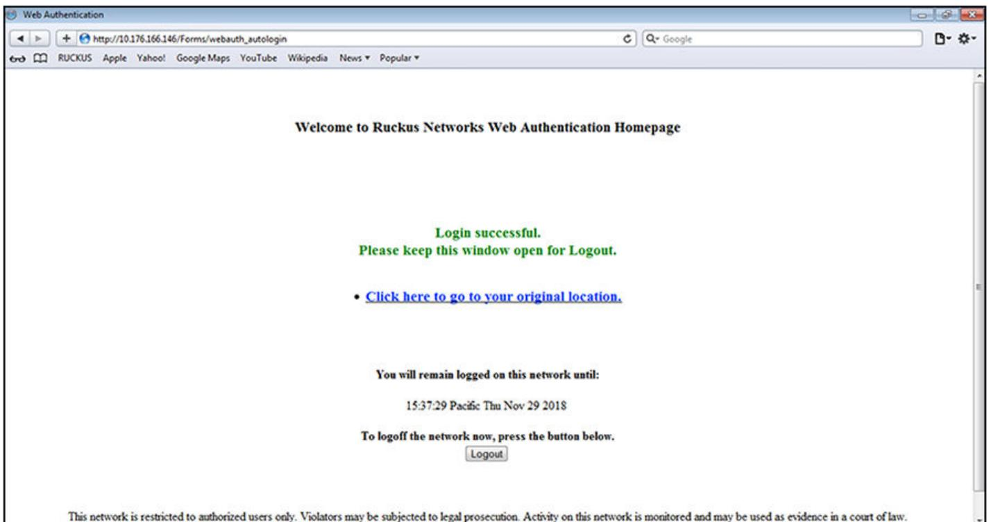
Once a host is authenticated, that host can manually de-authenticate by clicking the Logout button on the login success page. The host remains logged in until the re-authentication period expires. At that time, the host is automatically logged out. However, if a re-authentication period is not configured, the host remains logged in indefinitely.
