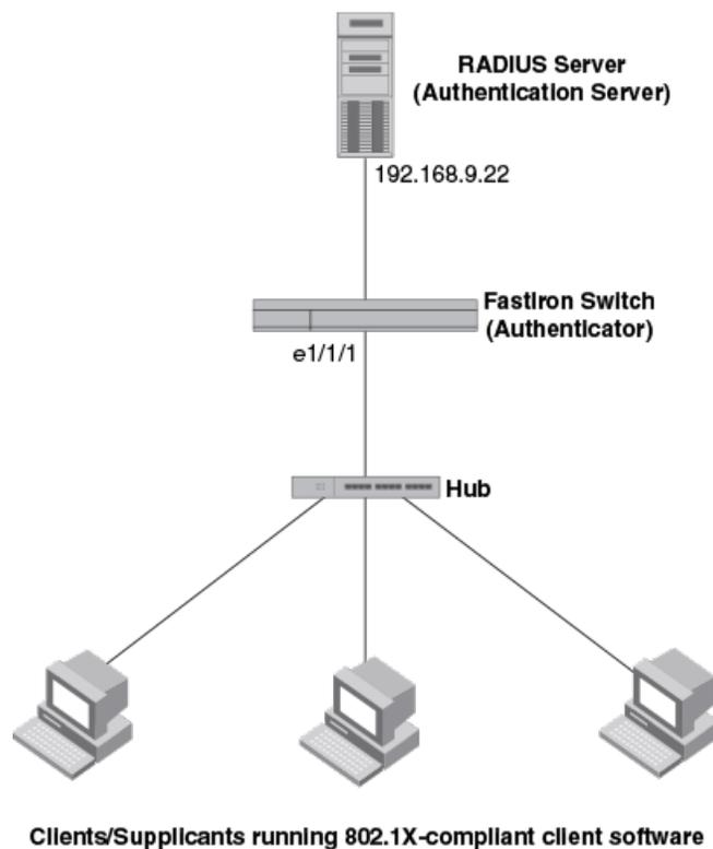
If multiple hosts are connected to a single 802.1X- or MAC authentication-enabled port, the ICX device authenticates each of them individually. Each host authentication status is independent of the others, so that if one authenticated host disconnects from the network, it has no effect on the authentication status of any of the other authenticated hosts.
