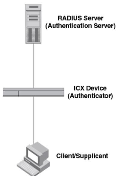
**Authenticator:** The device that controls access to the network. In an 802.1X configuration, the ICX device serves as the authenticator. The authenticator passes messages between the client and the authentication server. Based on the identity information supplied by the client and the authentication information supplied by the authentication server, the authenticator either grants or does not grant network access to the client.
