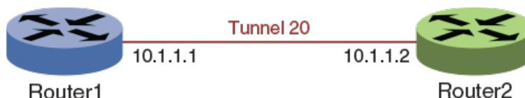
In the following example, Router1 and Router2 are the devices at each end of the tunnel. On each device, an IPsec profile (profA) is created and bound to the VTI by using the **tunnel protection ipsec profile** command.
