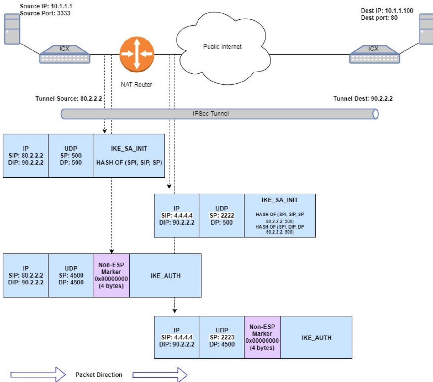
On the other side, again the hashes of IP address and port are calculated in the packet header. The re-calculated hashes are compared with the hashes received as part of the NAT-D payload. If they are different, it means the packet has undergone NAT. After this negotiation, the IPsec tunnel is established with UDP encapsulation. In UDP, both source and destination ports are set to 4500.
