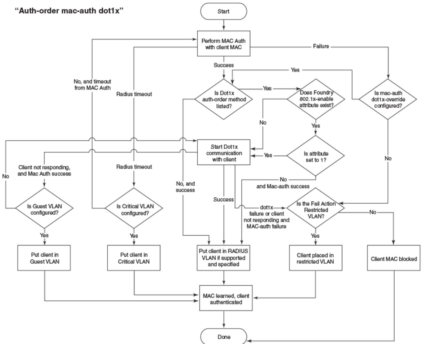
The following list describes how Flexible authentication works in various success, failure, timeout, and dynamic VLAN assignment scenarios:
