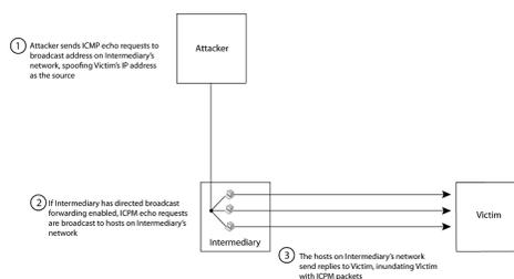
The attacker sends an ICMP echo request packet to the broadcast address of an intermediary network. The ICMP echo request packet contains the spoofed address of a victim network as its source. When the ICMP echo request reaches the intermediary network, it is converted to a Layer 2 broadcast and sent to the hosts on the intermediary network. The hosts on the intermediary network then send ICMP replies to the victim network.
